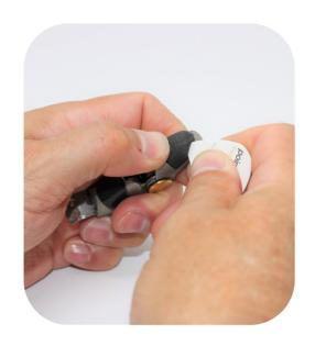
2. With the pad partially pried up, use your fingers to grab the pad and pull it the rest of the way out.
