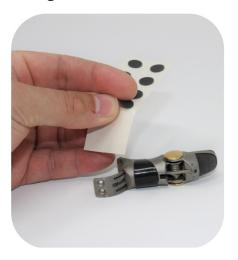
**3**. Center over the joint, then press on to the Chicago Bolt and hold pressure for at least 10-20 seconds. Clamping the pad down for 72hrs will yield optimal results, but is not necessary.
