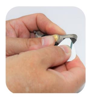
**3.** With the edges pressed in, apply pressure to the top of the pad and rock back and forth gently to help make sure the pad is fully seated. If the pad looks to be bulging out still, repeat Step 2.
