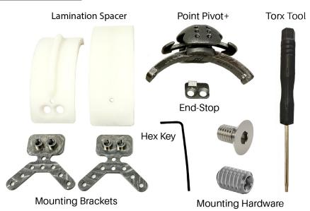
The **Point Pivot**+ comes assembled as one unit and is comprised of a curved track, carriage, shell, paddles, and several other internal parts. The curved track has 4 mounting holes. Additionally, an end-stop is included in the mounting kit and becomes part of the final system during the installation process.
