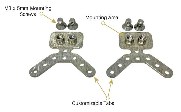
The mounting bracket is comprised of a mounting area and tabs that can be cut and shaped as desired. 2 mounting brackets are provided in each mounting kit.
