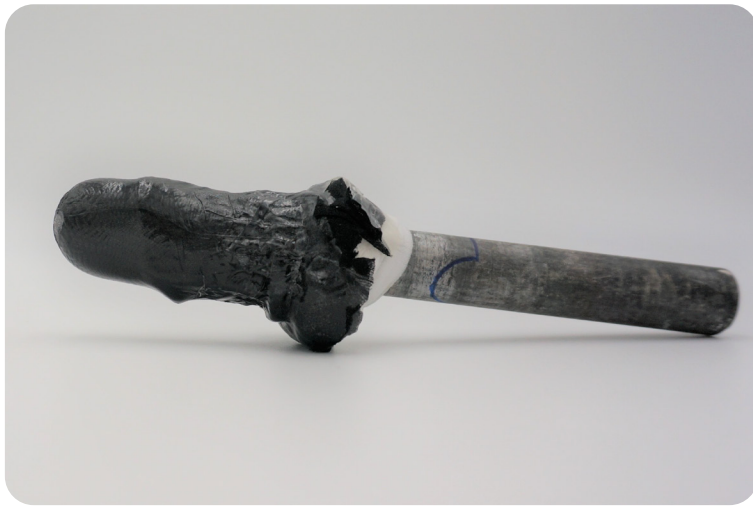
Initial layup attached to a mandrel
