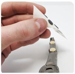
**3**. Center over the joint, then press on to the Chicago Bolt and hold pressure for at least 10-20 seconds. Clamping the pad down for 72hrs will yield optimal results, but is not necessary.
