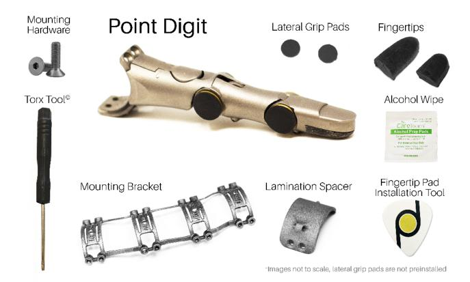
The **Point Digit** is a passive (i.e. not powered) mechanical finger for people with partial hand amputation. It features a ratcheting mechanism that enables one-handed use and up to 11 distinct locking positions. The **Point Digit** features integrated compliant touchscreen compatible\* fingertip pads for enhanced grip. The **Point Digit** is made from titanium for ample strength.
