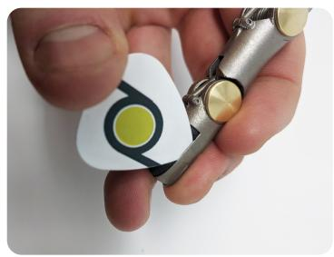
**3.** With the edges pressed in, apply pressure to the top of the pad and rock back and forth gently to help make sure the pad is fully seated. If the pad looks to be bulging out still, then repeat Step 2.
